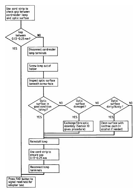
Fig. 6.3 Flow chart algorithm for a maintenance procedure.
