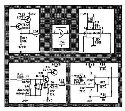
Fig. 10.36 Block circuit diagram supported by block text shown in Fig. 10.35 (reproduced by permission of S.W.Amos from Wireless World).
